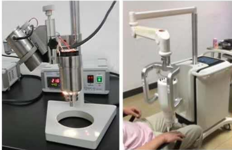
FIGURE 2 Local hyperthermia device (on the left is the old device and on the right is the new version). The yellow light source of the treatment head provides heat, and the infrared point monitors the real-time temperature (the red number in the upper part of the display). The host will adjust the real-time temperature of the treatment target to the set temperature (yellow number in the lower part of the display), based on the temperature feedback of the infrared point. The new device can provide more precise treatment temperature, with a smart touch-screen console that sets temperature and treatment time for different patients and treatment sites.
